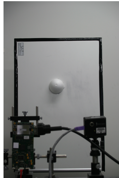
Fig. 8. Measured space with a hemisphere and a white planar board.
