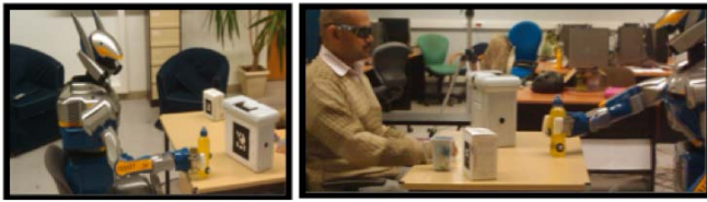
Fig. 10. Making the bottle accessible to the human, (a) Grasping the bottle by planning collision free path (b) final place where the robot is putting the bottle so that human can access it.
