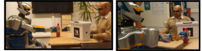
Fig. 13. Hiding the bottle from the human. (a) Initial position of bottle, (b) final position of the bottle hidden from human.
