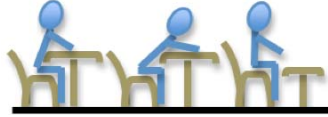
Fig. 4. Human closer to the table (a), could lean less compared to sitting away from the table (b). Table is too low to be reached without leaning (c).
