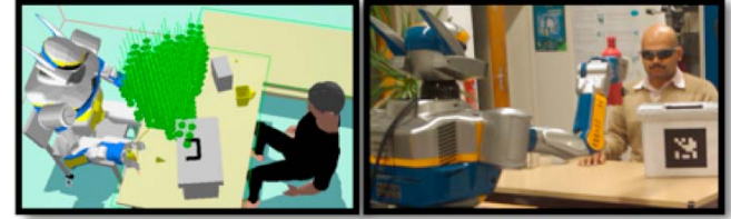
Fig. 12:(a) Candidate points in 3D to show the bottle, which was actually hidden from human (b) Robot showing the bottle at the feasible place.
