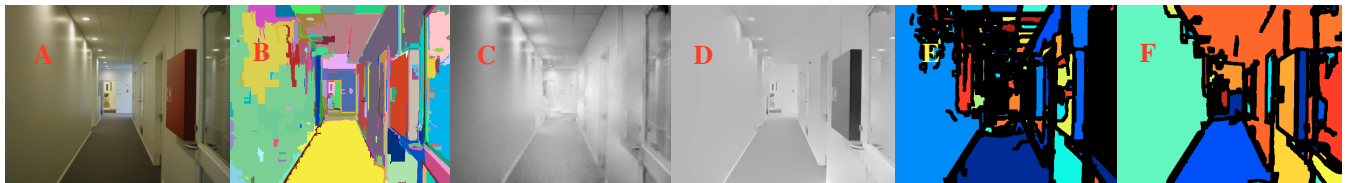
Figure 1. Intrinsic Image Extraction and Segmentation (A) Input color image (B) Segmentation using the standard Felzenszwalb-Huttenlocher (FH) graph based algorithm – demonstrates high clutter in regions of the left wall with lighting changes (C) Shading intrinsic image (D) Reflectance intrinsic image – note that C and D (obtained by inversion of input image gradients classified as shading or reflectance respectively) are presented here only to demonstrate the separation of shading/lighting effects from material properties; segmentation is not carried out on these images (E) Segmentation on the input image using a low complexity multi-scale full gradient edge analysis scheme (F) Segmentation on the input image with the same scheme using reflectance-only gradients – shows superior performance in wall regions affected by lighting changes in comparison with full-gradient image segmentation schemes such as the graph based FH. Note that similar values of gradient and region size thresholds were used for the two approaches - FH and our scheme.
