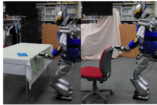
Fig. 10. Left: Pushing a static obstacle (table), Right: Pushing a movable obstacle (chair)
