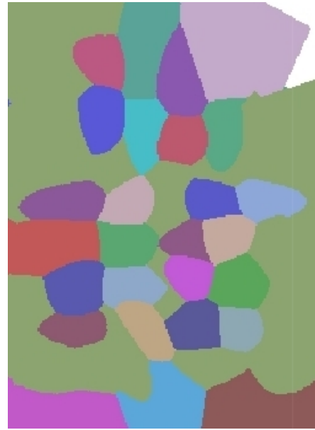
Fig. 6. A visualization of the decision boundaries of the regions representing the rooms and hallways on the map shown in 4. All the Gaussians are colored in different colors for identification. This figure is best viewed in color.
