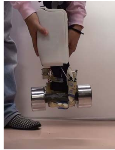
Fig. 9. The system holds up five-kilogram weights.
