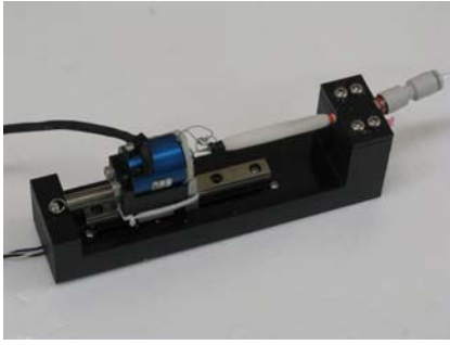
Fig. 9. Experimental setup for estimation the model of McKibben pneumatic artificial muscle
