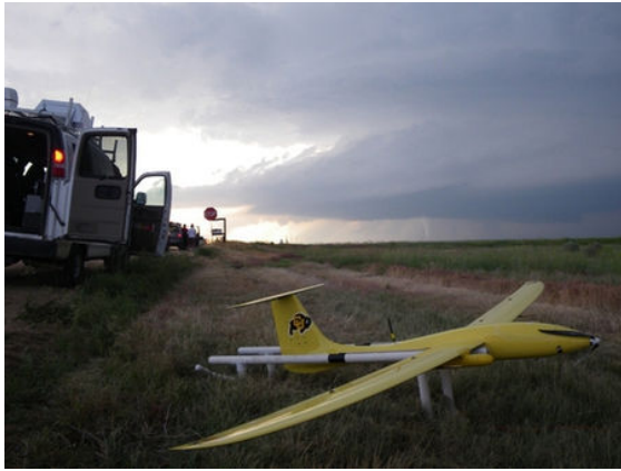
Fig. 2. The Tempest UA pictured ready for deployment into the tornadic supercell pictured in the background. Photo taken during the Spring 2010 campaign of the VORTEX2 experiment.
