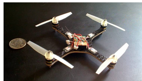
Fig. 13. The mini quadrotor developed by Daedalus Flight Systems and UMD uses the GINA hardware, but modifies the firmware to include an onboard attitude stability loop to control its four brushless DC motors.
