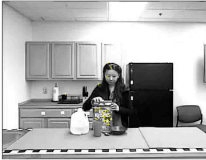
Fig. 3. Frame of the SIFT features extracted during recognition. These key points are then compared with the key points saved in each object dictionary.
