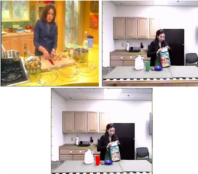
Fig. 12. Color segmentation results, colored in with red, used in color and shape features used by MCOR. Top left shows the segmentation of the knife, top right shows the segmentation of the cereal box, and bottom shows segmentation of a cup. Note the better segmentation of the homogeneous colored knife and the less precise segmentation of the more textured cereal box.
