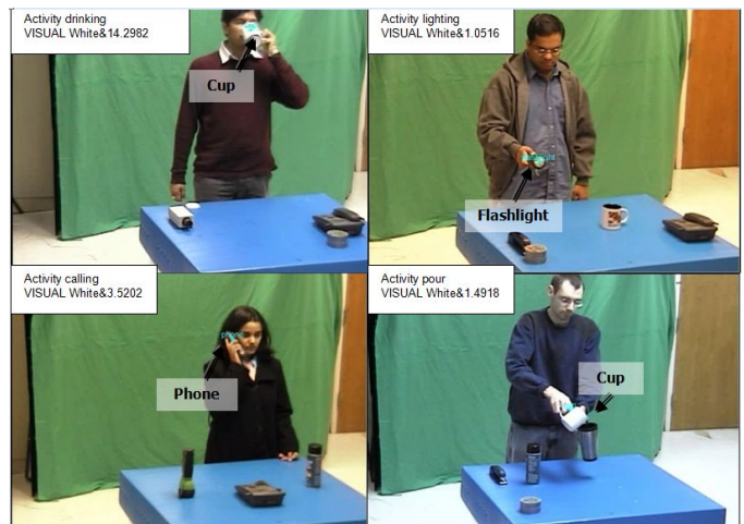
Fig. 7. Captured frames taken from results video generated after processing various video clips from the Gupta and Davis Dataset. Each frame shows the point in the video when an activity cue was recognized, which allowed for the object being used to be recognized and the color and shape information (top right of each frame) to be stored.
