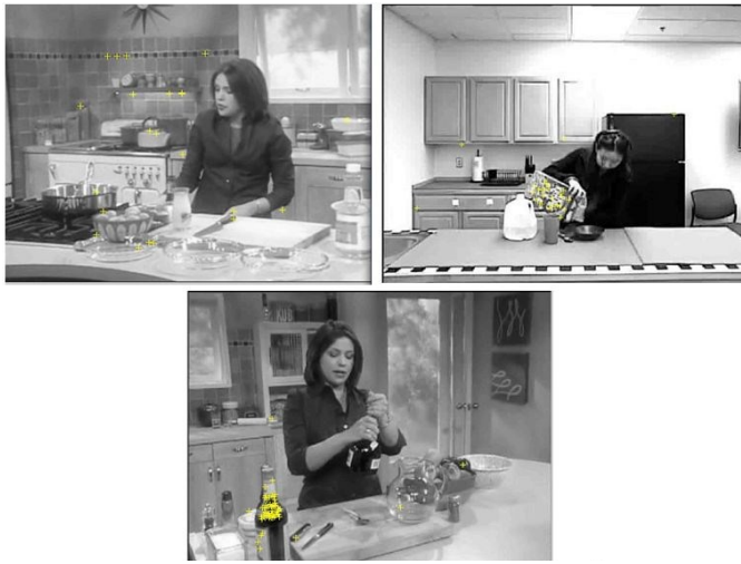
Fig. 11. SIFT features, represented by yellow + signs, found to match the model of the knife (top left), the cereal box (top right), and the wine bottle (bottom). Note the large number of matched SIFT features for the cereal box because its large amounts of texture, and the small number for the less textured knife.
