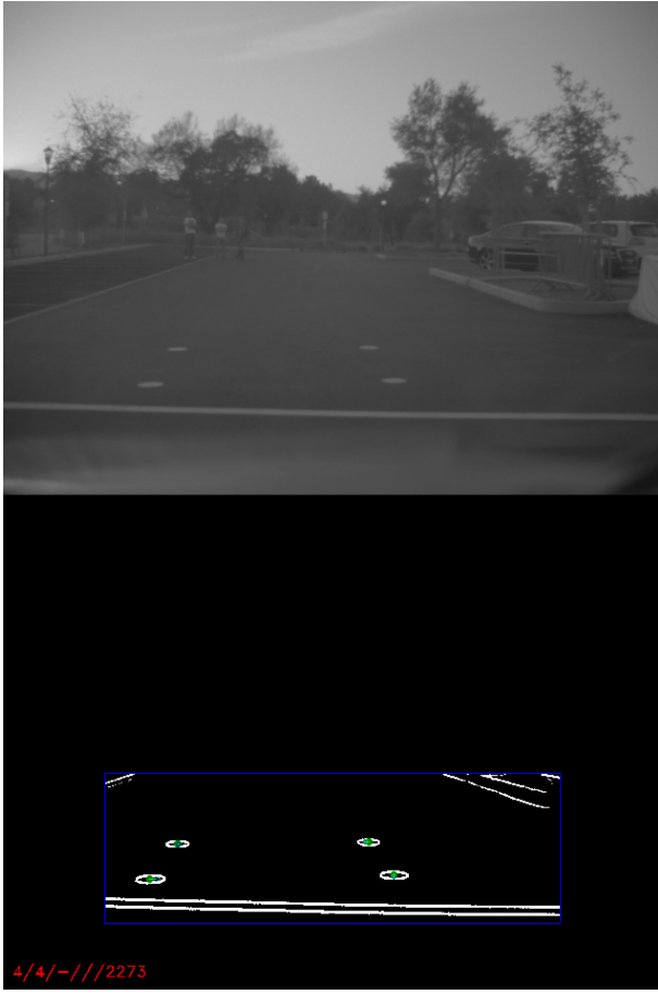
Fig. 4. The raw camera image (above) is pre-processed with morphological operators (below). An ellipse detector recognizes markers from this image.
