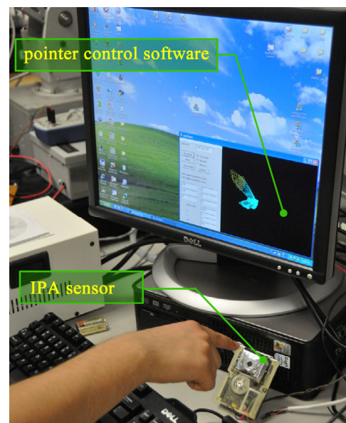
Fig. 1. T-less : The proposed touch less user interface by using IPA
