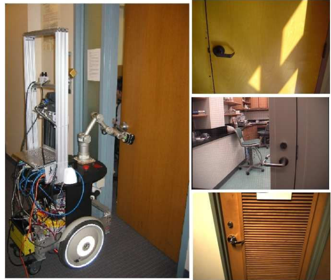
Fig. 1. STAIR robot opening a novel door and images of the types of doors used in our experiments.
