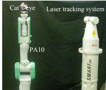
Fig. 3. Experimental setup for measuring position of robot arm's tip
