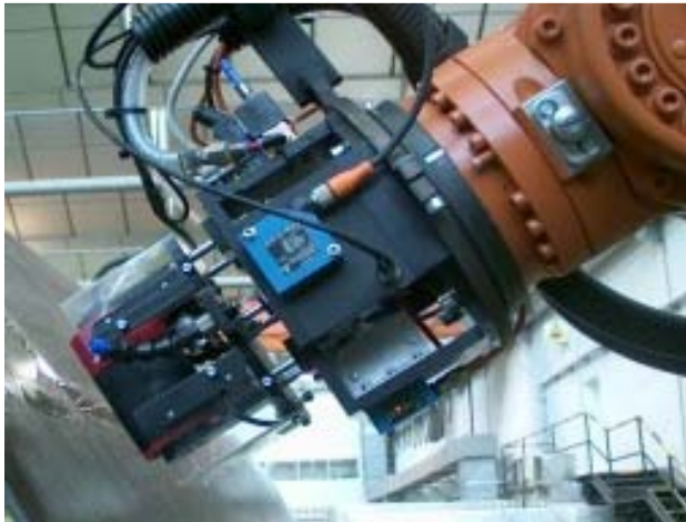
Fig.3. Inspection sensor place at the end robot effector. Four laser are used to measure the distance between end robot and the surface inspected
