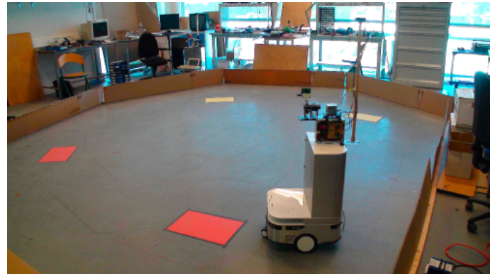
Fig. 1. The robot in its environment (5m x 5m). A color detector is placed under the robot. Colored squares on the ground represent simulated resources.
