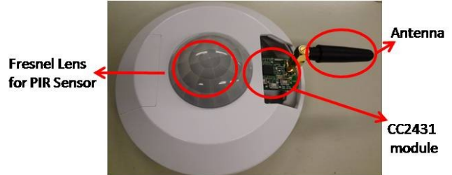
Fig. 4 The experimental platform integrated with CC2431 and pyroelectric sensor
