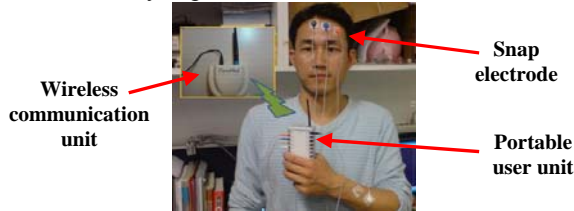
Fig. 7 EMG measurement setup.
