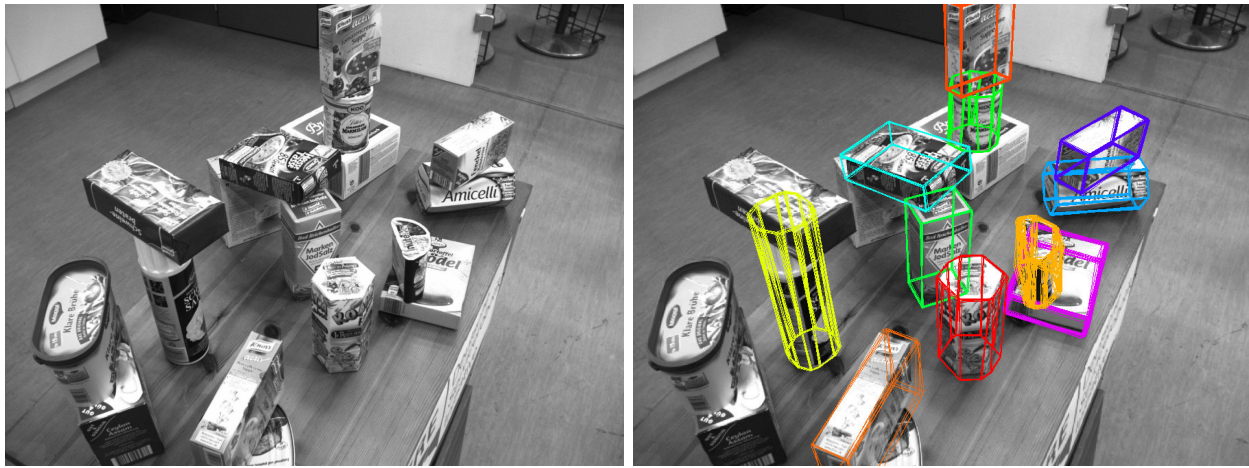
Fig. 7. A complex scene composed of several household objects in various configurations. In the left image samples drawn from the observation model p(z|x) were overlaid onto the source image (colors indicate object class IDs; not relevant here).
