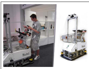
Fig. 1. The Interactive Behavior Operated shopping Trolley (InBOT). It is equipped with a mecanum drive for full holonomic movements and the environment is observed by two laser range finders. Additionally the user can find a wide range of equipment for interaction with the robot. The setup is described in [6]. The left hand side shows a scene from a user study.
