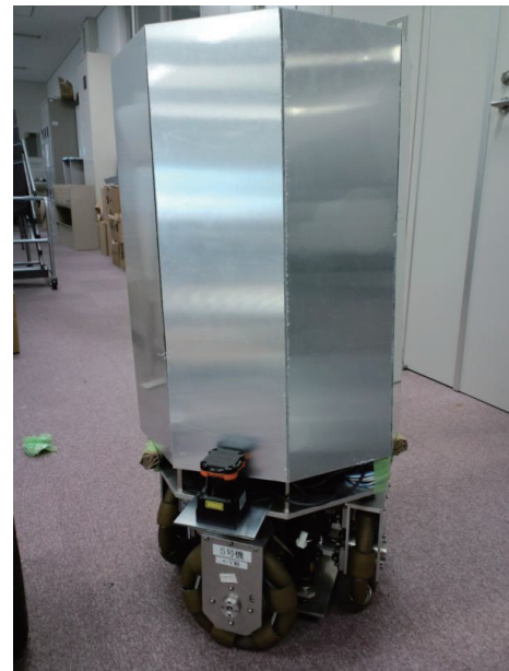
Fig. 9. Appearance of the omni-directional robot
