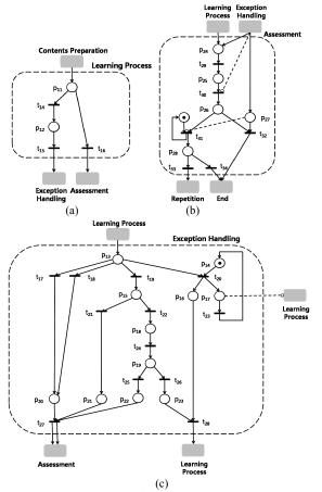
Fig. 5. The Petri nets of the modules at the processing stage in r-learning (a) Learning Process (b) Assessment (c) Exception Handling
