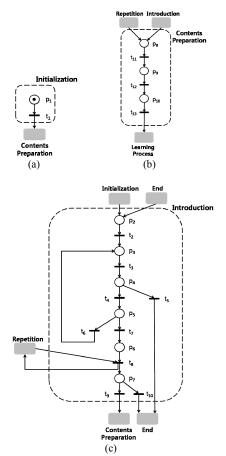
Fig. 4. The Petri nets of the modules at the preparing stage in r-learning (a) Initialization (b) Contents Preparation (c) Introduction
