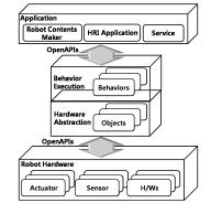
Fig. 8. The application of Open API to a robot software platform
