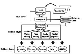
Fig. 2. The three-layer architecture of the behavior-based control system for operating an intelligent tutor robot
