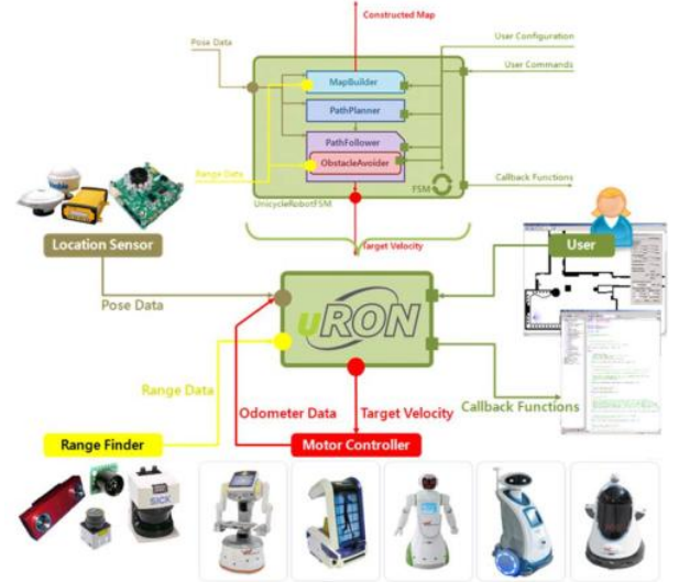
Fig. 3. System architecture of uRON
