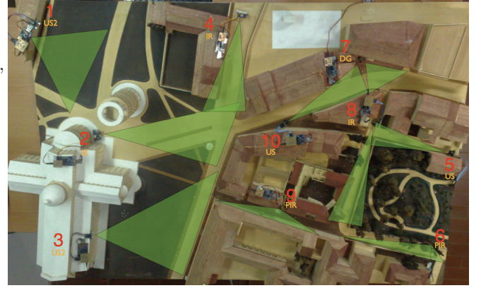
Fig. 1. Scale model of the area nearby Pisa’s Leaning Tower. Green cones represent the visibility areas of every agents.
