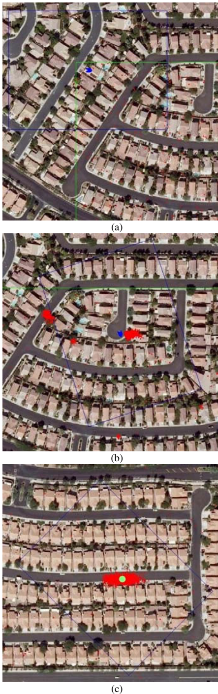
Fig. 4. The result of performing Monte Carlo Localization of a UAV on a sample image taken from Las Vegas, Nevada, during different steps. a) initial step: particles are uniformly distributed; b) a middle step (step 80): many different hypotheses coexist; c) last step (step 100) only two hypotheses are remained, and the best one is closer to the true pose. The red dots are the particles, the green arrow-like ellipse indicates the true pose, and the big green circle shows the estimated pose based on particles. The blue and green rectangles are window viewed by the camera in each step, and the acceptable region for particle generation and resampling in all steps.
