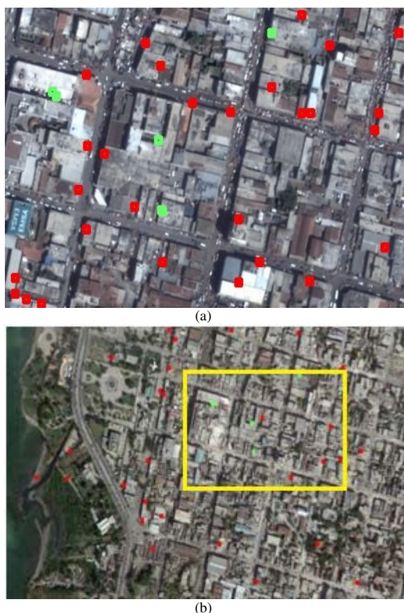
Fig. 1. The found matched pairs in two images of Port-au-Prince, Haiti. a) An image taken before the earthquake, and b) the image of the same region with its neighborhood, taken after the earthquake. The green marks show the correct matched SIFT feature pairs, whereas the red marks indicate incorrect matched pairs.
