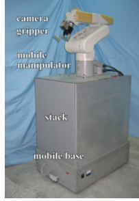
Fig. 1. Developed mobile manipulator.
