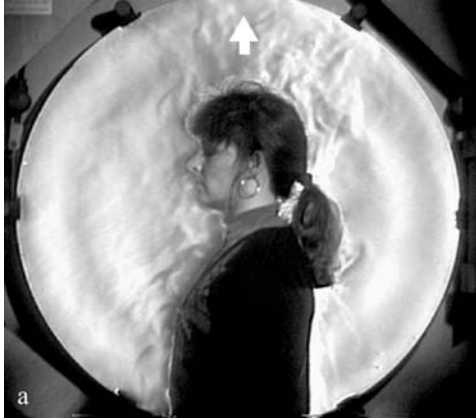
Figure 1. A Schlieren photograph visualising heated air rising from the human body. (courtesy Prof. G. Settles, Penn State University)
