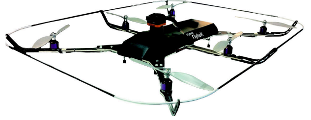
Fig. 5. Flybox UAV in the hexacopter configuration.
