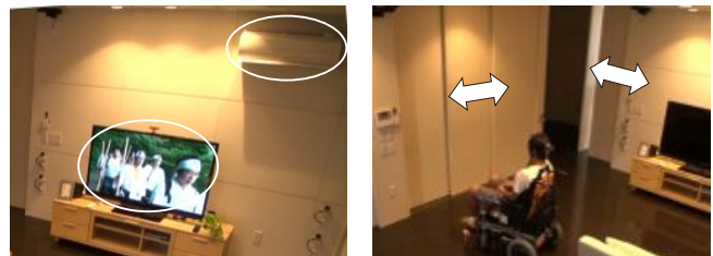
(e) Household electrical appliances are controlled from the server. (f) Doors are controlled according to the navigation plan.
