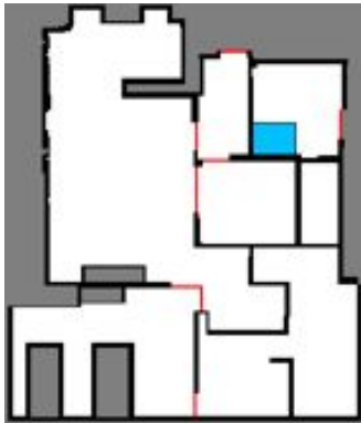
Fig. 7. Grid map of the smart living environment. Doors are represented in thin red lines and the elevator in light blue.
