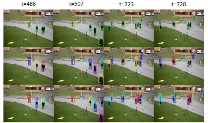
Fig. 6. Tracking results of the ‘PETS2009’. First row: detection results. Second row: tracking with the STS . Third row: tracking with the ITS .
