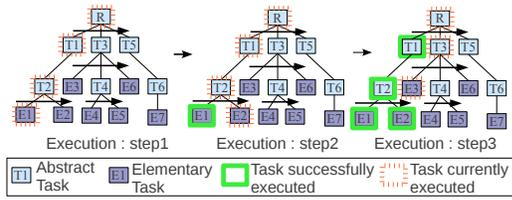
Fig. 3: Execution of an iHTN: HiDDeN processes root task  $R$ , descends to task  $E1$ . When  $E1$  is successfully achieved, the following task is  $E2$ , then  $E3$ , and so on as long as no fault is detected.
