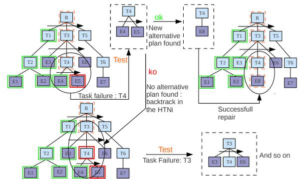
Fig. 4: The repair process: elementary task  $E5$  fails, which implies a repair of task  $T4$  (top, left). If a new plan is found, the iHTN branch is replaced (top, right); otherwise, the repair process is applied to  $T3$  (bottom).
