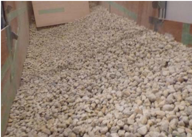
Fig. 11. Simulated volcanic field covered with pumice stones. The slope angle can be changed manually using a shovel.
