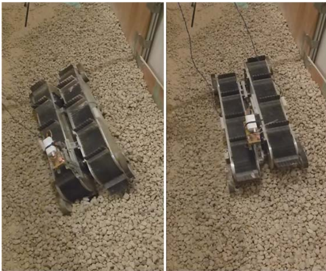
Fig. 13. Photographs of indoor experiment with slope angle of 30^\circ . Robot in the normal contact configuration (left), and in the horizontal contact configuration (right).
