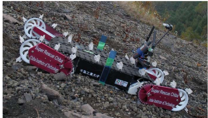
Fig. 1. Quince version for volcanoes: Originally developed for rescue applications, it consists of two main tracks and four subtracks. It is equipped with a total of six mounted actuators.
