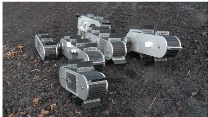
Fig. 2. Novel design of tracked vehicle ELF, which consists of two main tracks and four subtracks. It is equipped with a total of eleven mounted actuators that give it a high degree of traversability on weak and uneven terrains.
