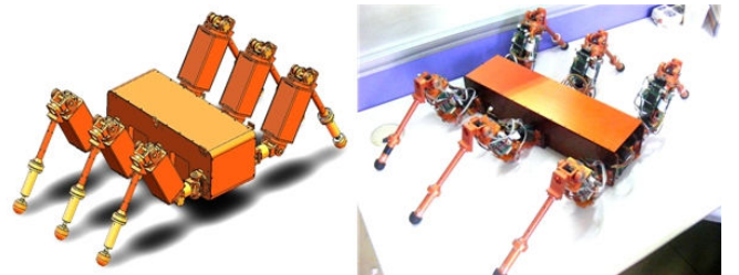
Fig. 9. The hexapod robot: CAD model (left) and physical prototype (right)
