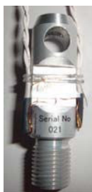
Fig. 7. (Left) Inline tension sensor (Right) Calibration results for three sensors
