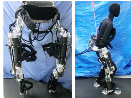
Fig. 1. ATR hybrid drive eXoskeleton Robot (XoR) Prototype 2: (Left) Front view, (Right) Side view with mannequin.
