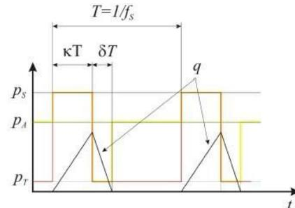
Figure 4. Flow control mode
