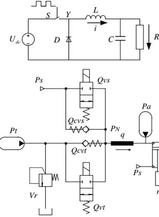
(A) Electronic buck converter (B) Hydraulic buck converter
