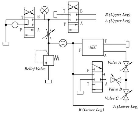
Figure 7. Schematic of the Test System
