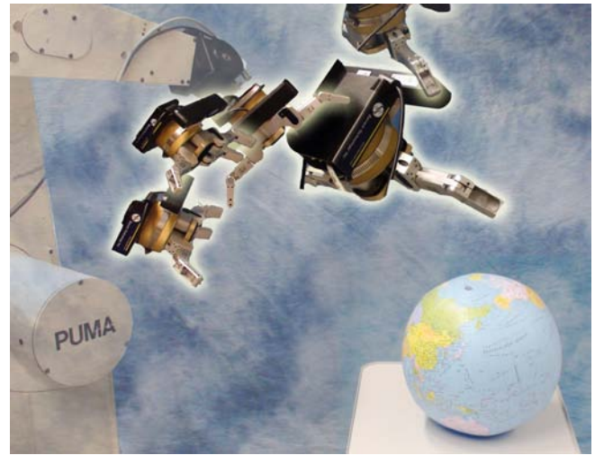
Fig. 7: The experimental setup for the simple environmental constraints: The sensor observes the object from the five different perspectives shown.
