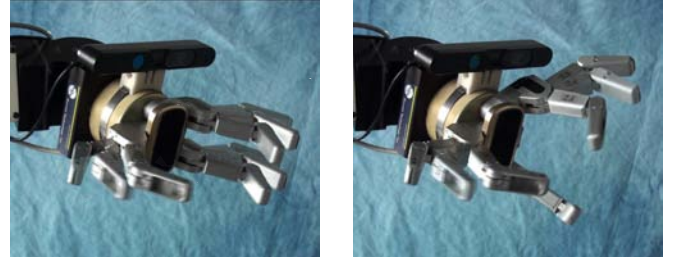
Fig. 1: The motion of two different preshapes of the Barrett Hand. To find suitable grasps we search for structure that is shaped complementarily.
