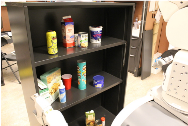
Fig. 6: Experimental setup. The PR2 with a head-mounted Kinect views the objects on a shelf from the front. The task is to search for a target object by rearranging other objects on the shelf.
