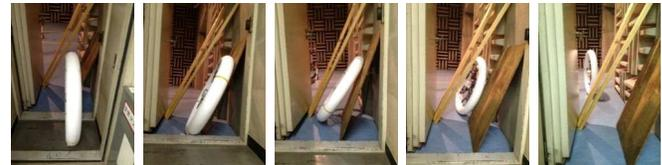
Fig. 2. Example of mono-wheel mode in the field in a disaster. The robot is able to pass through narrow vertical-diagonal gaps with an inclined rolling motion.
