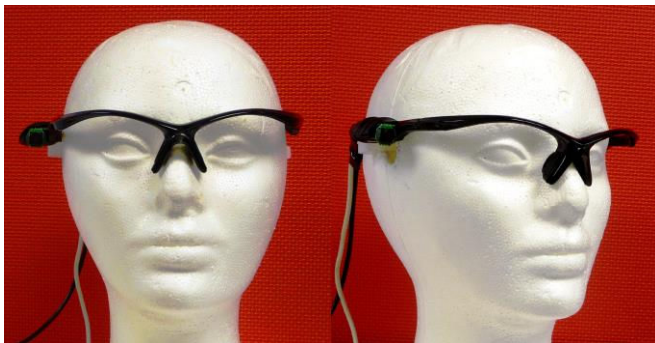
Figure 2. Design of the eyeglasses. The sensors are attached to the left earpiece
