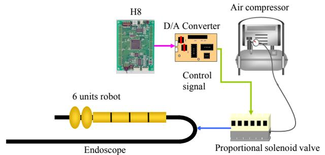
Figure 5. Control system of the pneumatic robot.
