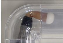
(a) Head unit colliding with a narrow elbow.
