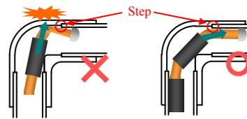
Figure 20. Image after the head section has climbed over the step.
