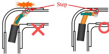
Figure 19. Head section climbing over a step.
