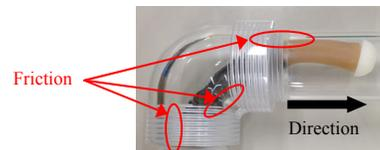
Figure 11. Image of a robot passing through an elbow.
