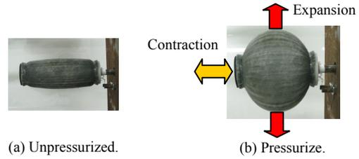
Figure 4. Straight-fiber artificial muscle.
