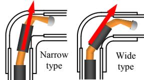
(b) Effect of elbow type on approach angle.
