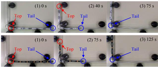
Figure 18. Passage time of each robot in a horizontal elbow.
