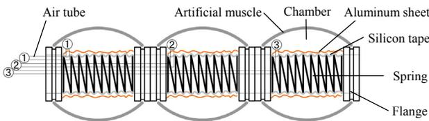
Figure 3. Structure of a peristaltic crawling robot.
