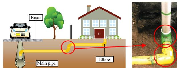
Figure 1. Common configurations of 1-inch gas pipes.
