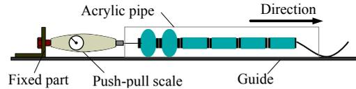
Figure 16. Experimental setup for measuring frictional force.
