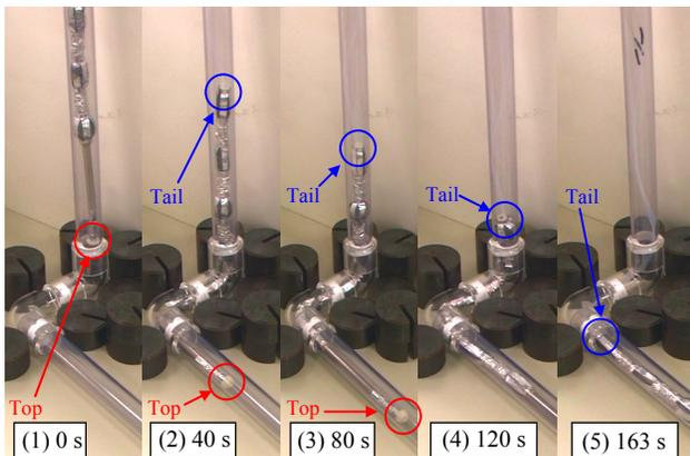
Figure 24. Experiment in continuous elbows.
