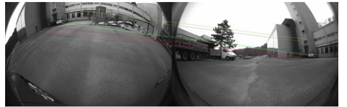
Fig. 7: The subset of the same feature point correspondences that correspond to 3D scene points in the maps.
