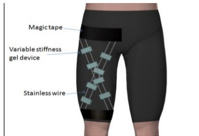
Figure 11. Structure of the designed variable stiffness gel spats.
