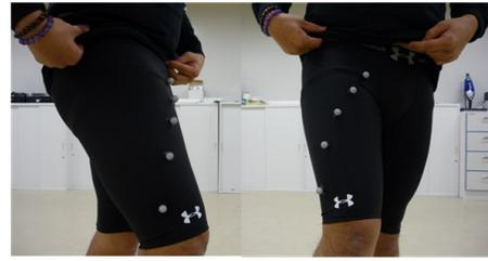
Figure 13. Arrangement of markers to capture motion.
