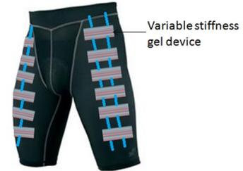
Figure 9. Structure of the variable stiffness gel spats.
