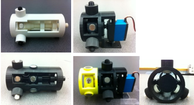
Fig. 10. Two prototypes of magnetic brake are built. Prototypes verify the ability of the mechanism to produce controllable normal force while consuming very little energy.
