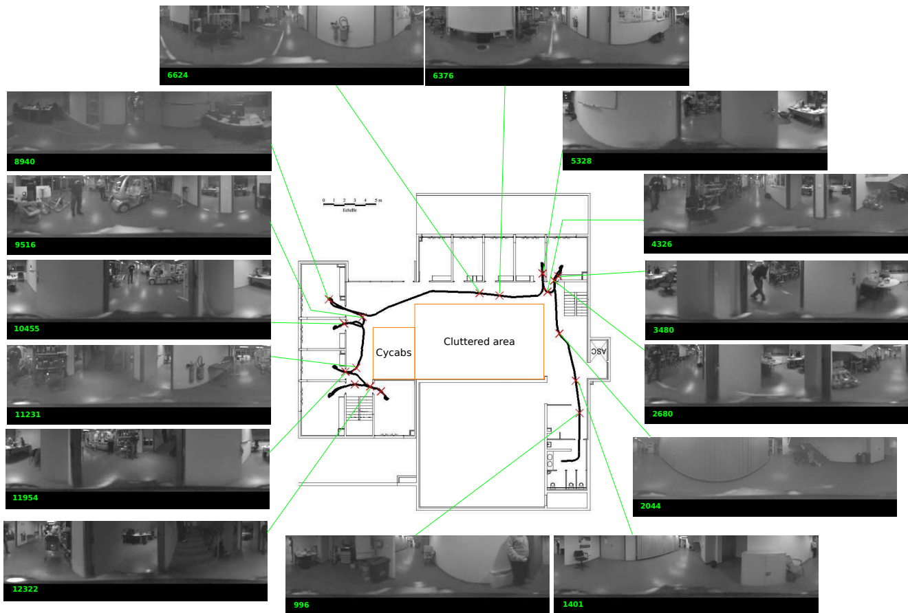
Fig. 6. Indoor trajectory inside the Robotic Hall. Detected change-points are marked with red crosses.
