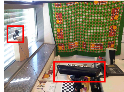
Fig. 1. Illustration of the experimental setup. The RGB-D sensor is on the bottom of the image while the RGB camera is on the left side.
