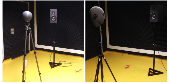
Fig. 6. Experimental setup. (Left) Spherical head mounted on the tripod, facing the loudspeaker emitting the considered sound. (Right) KEMAR head in the same conditions.
