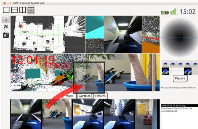
Fig. 3. Dragging a thumbnail loads a picture in a visualization panel. Clockwise from top-left: a 2D top-down view, the robot's front camera, the 3D reconstructed scene, and a picture from a mobile device. Here, the mobile picture helps climbing the stairs more than other views.
