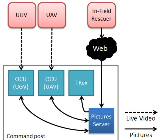
Fig. 2. The system architecture with the In-Field Pictures Server
