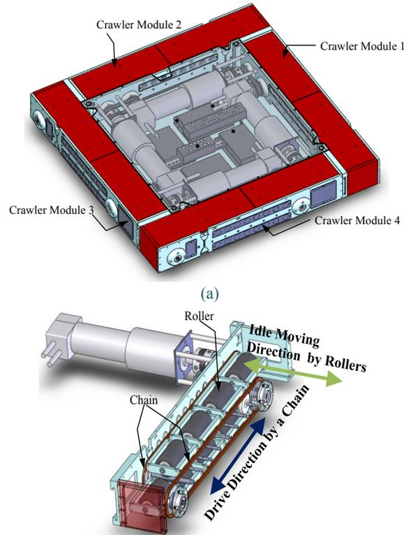
Fig. 3. Structure of the horizontal driving mechanism. (a) Overview. (b) Crawler module of the horizontal driving mechanism.
