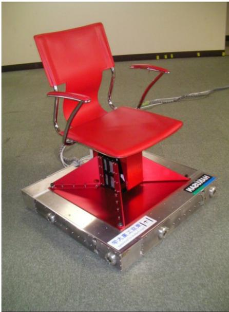
Fig. 7. Prototype of Jishin-The-Vuton 3D. Air cylinder (model: MB1 series, bore size:  $100 \text{ mm}$ , maximum operating pressure:  $1.0 \text{ MPa}$ , stroke:  $50 \text{ mm}$ , manufacturer: SMC). Electro-pneumatic regulator (model: ITV3000series, regulating pressure range:  $0.005$  to  $0.9 \text{ MPa}$ , manufacturer: SMC). ( $+25 \text{ mm}$ ).
