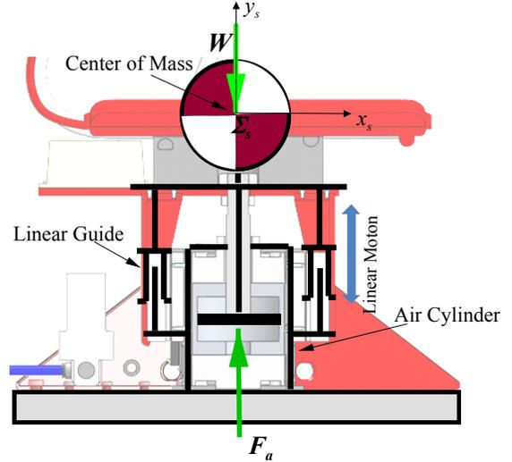
Fig. 6. Schematic diagram of the vertical driving mechanism.
