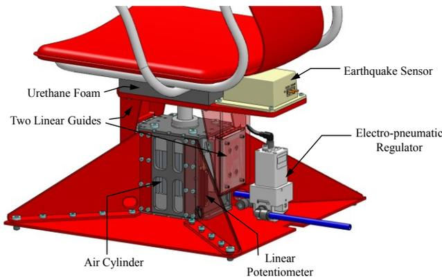
Fig. 5. Components of the vertical driving mechanism.
