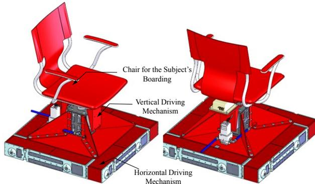
Fig. 2. Structure of Jishin-The-Vuton 3D.
