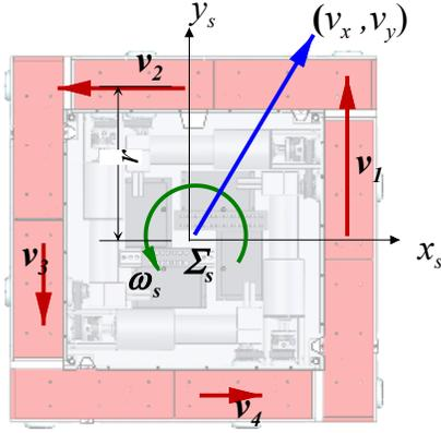
Fig. 4. Schematic diagram of the horizontal driving mechanism.
