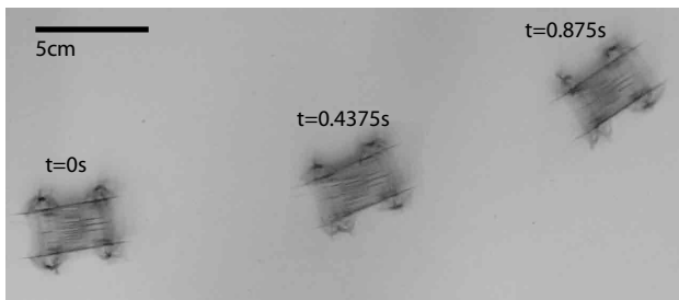
Fig. 12. By exploiting HAMR-VP's high bandwidth and quality factor powertrain, speeds up to 37 cm/s (8.4 body length per second) have been achieved using gait frequencies up to 70Hz.
