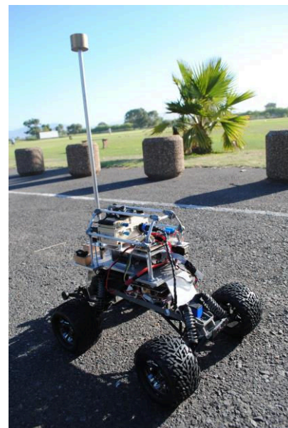
Fig. 2. Dima , the high speed actuated tail robot.
